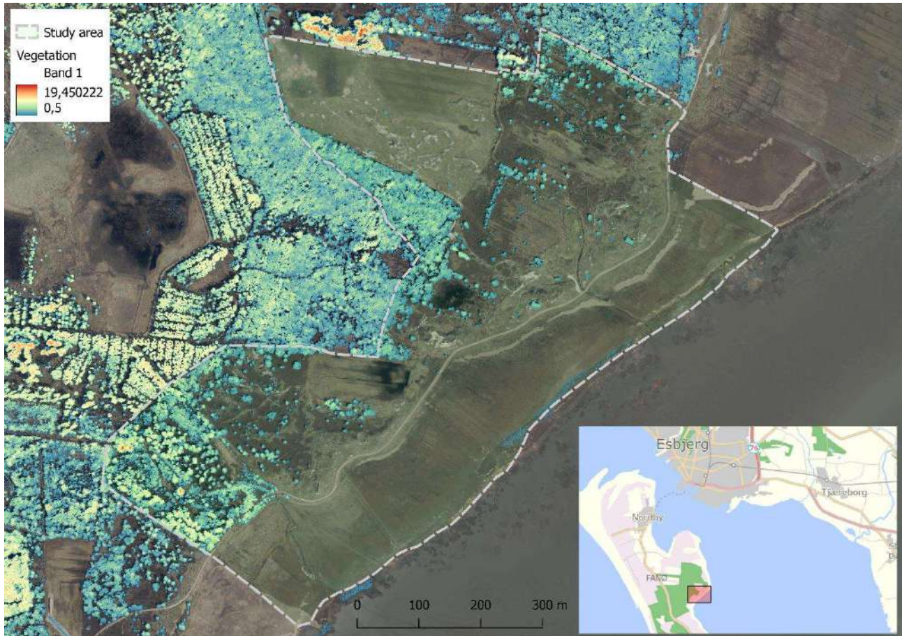
Figure 6: Bushes and trees registered in and around the study area. Blue colors are the lowest vegetation, then comes green, yellow, and red as the tallest vegetation, in relation to the terrain. The grey dashed line is the outline of the study area.
